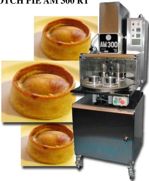
The Powerchampion AM300 RT Scotch Pie machine has an adjustable speed indexing table supporting 1 or 2 dies. The Die equipment has thermostatically controlled electric heaters and compressed air release system to prevent deformation of the product. AM300 RT model can run in either manual or continuous automatic mode depending on your requirement.
